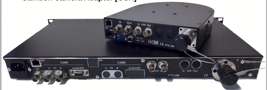
Cambox Control Unit [CCU] (single channel with 12G Option and SMPTE showed)
