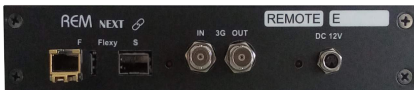
Fast & Standard FlexyBUS – Bidirectional SDI 3G Power OUT to energize devices (e.g.: PTZ)
